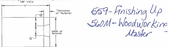
The angle for the PIns and Tails of the dovetail joint is 70-80 degrees.
